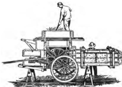
Belt power hay baling press in operation. May be operated by horse, steam, or gasoline power
